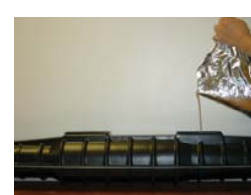
Pouring of polyurethane resin
